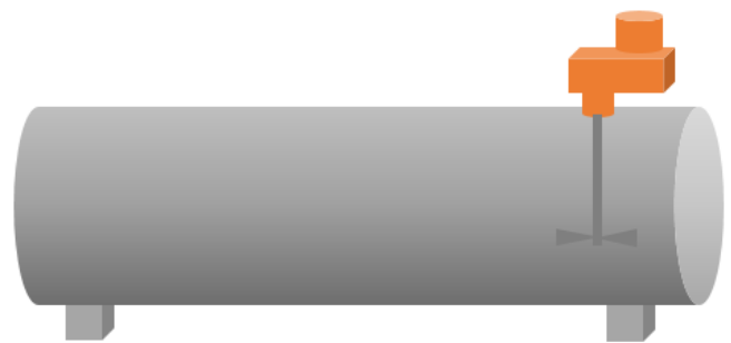
Figure 1. Even if the viscosity of the liquids you are blending is water-like, one industrial mixer placed at the end of a long, horizontal cylindrical mixing tank won't be effective.
